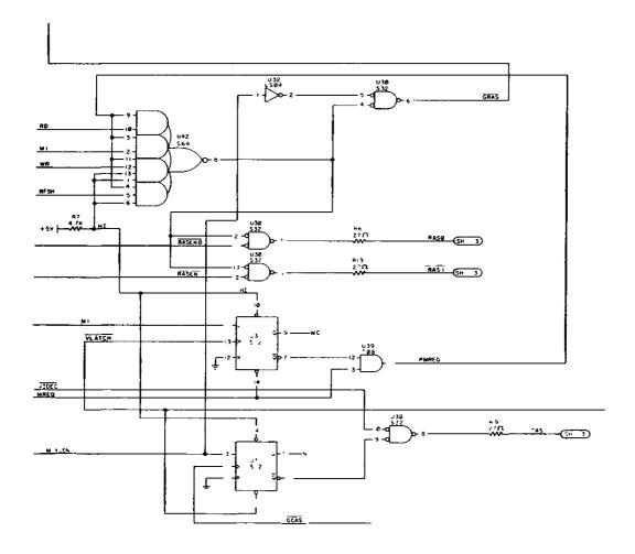
Figure 2-9. Video RAM and DRAM Timing Circuit. (Page 2 of Schematic)
