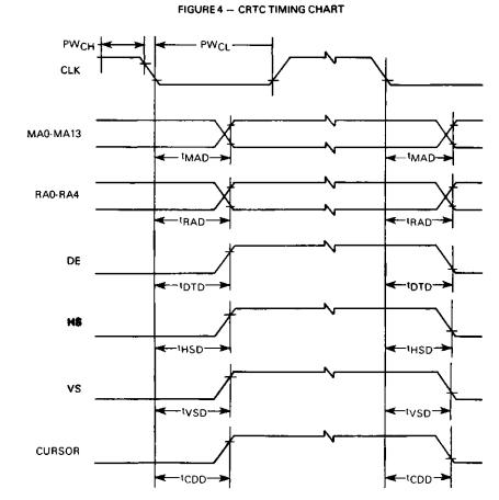
NOTE Timing measurements are referenced to and from a low voltage of 0.8 volts and a high voltage of 2.6 volts unless otherwise noted
