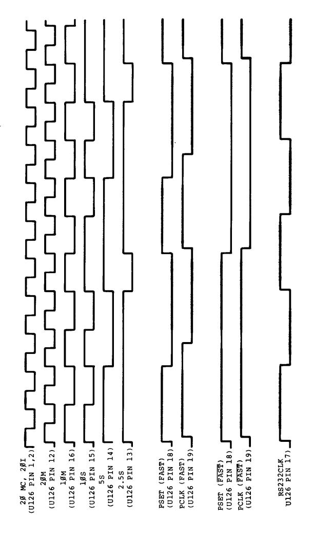
Figure 3-2. System Timing
