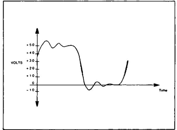
Figure 2. TYPICAL "RINGING" WAVEFORM from TTL INPUT
