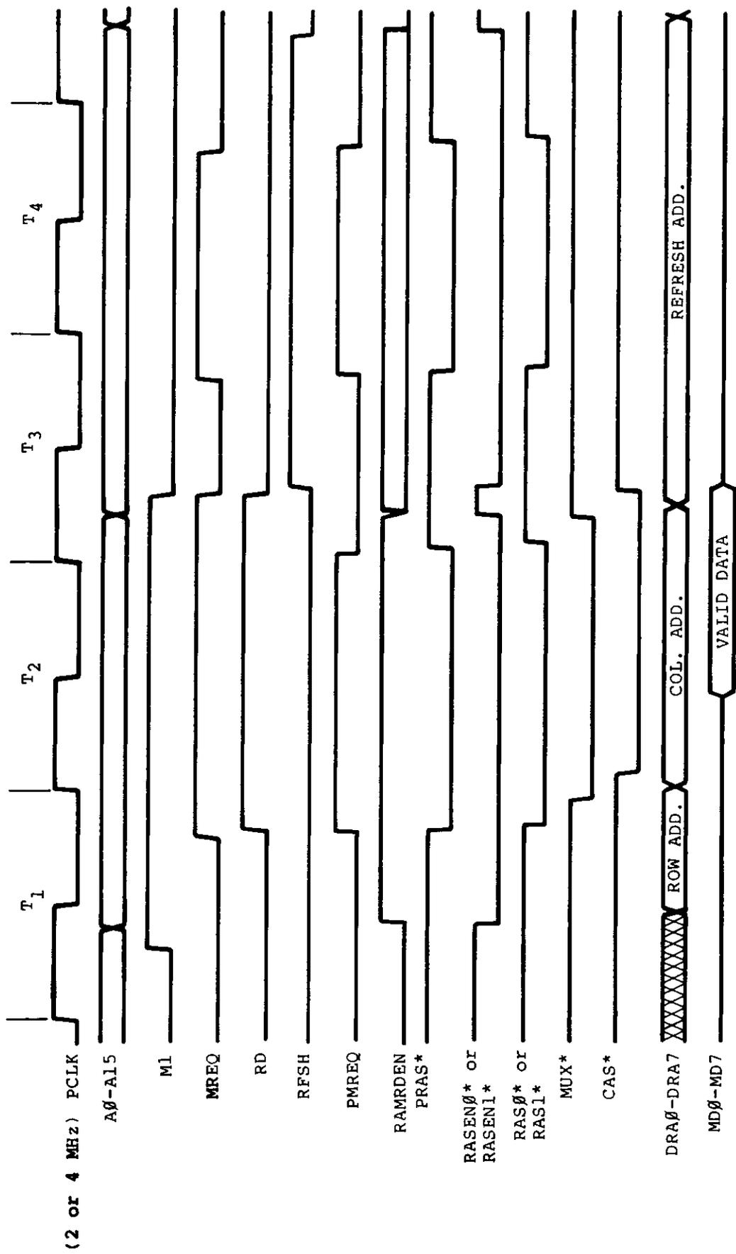
Figure 2-10. M1 Cycle Timing
