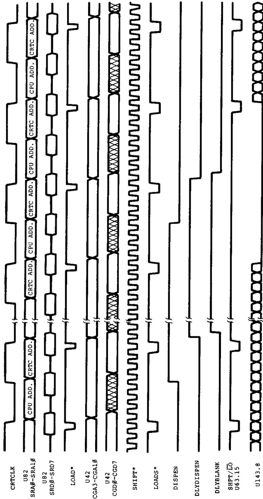
Figure 3-14. Video Blanking Timing
