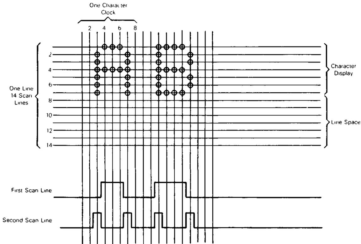
Referring to Figure 1, the MC6835 CRT controller generates the Refresh addresses (MA0-MA13), row addresses (RA0-RA4), and the video timing (vertical sync – VS, horizontal sync – HS and display enable – DE). Other functions include an internal cursor register which generates a Cursor output when its contents compare to the current Refresh address. A select input, PROG, allows selection of one of two mask programmed video formats (e.g., for 50 Hz and 60 Hz compatibility).
