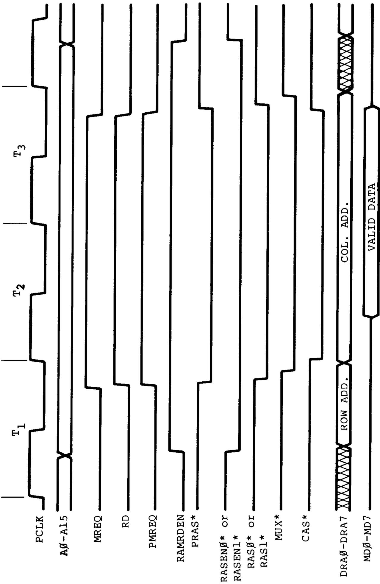
Figure 2-11. Memory Read Cycle Timing
