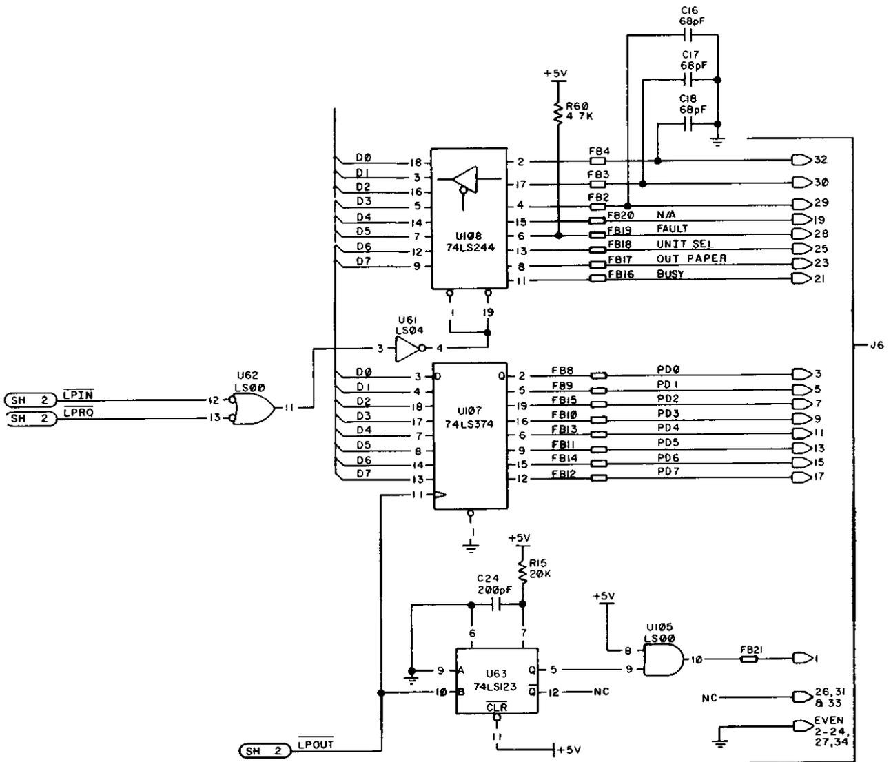
Figure 2-19. Printer Circuit
