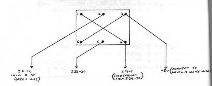
SWITCH CONNECTIONS FOR LEVEL II+I
