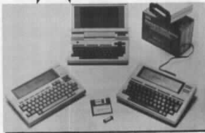
Custom Plug-in ROM's are available for Tandy Models 100, 102, 200, and NEC PC-8201 portable laptop computers.
