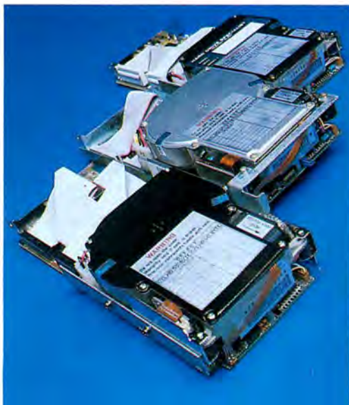
Not all hard disks will work in a 1000. These will. Left, 64MB drive from Megahaus; center, Tandy's 20MB drive; upper right, Hard Drive Specialist's 45MB drive (right).
