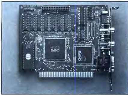
The Multi-EGA by Boca has a light-pen port and feature connector with two RCA video jacks.
