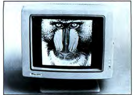
The Relisys RE5155 multiscan monitor features 800-dot by 560-line resolution.
