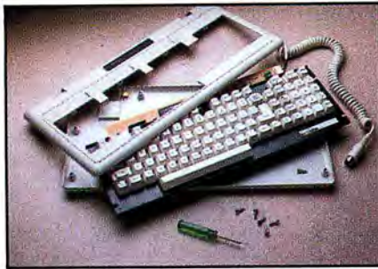
Photo 2. Separate the cover halves from the keyboard assembly.
