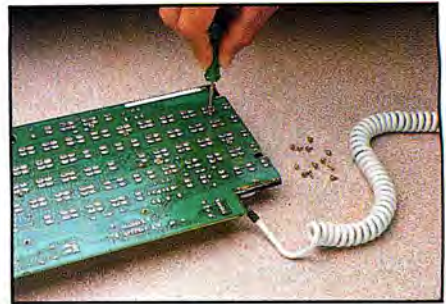
Photo 3. Remove the keyboard assembly from the printed circuit board.
