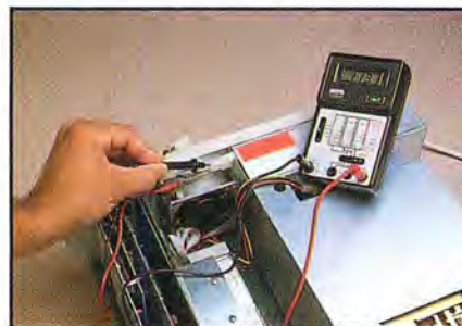
Photo 6. Measuring the voltage at the power plug to the fan.
