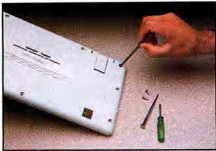
Photo 1. Remove the screws holding the keyboard cover together.
