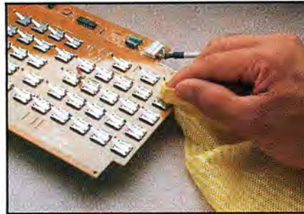
Photo 5. Use a moist cloth to clean the key contacts.
