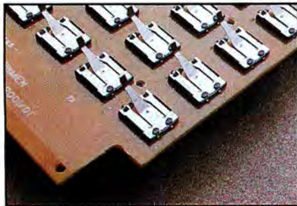
Photo 4. Metal contacts are underneath each key.
