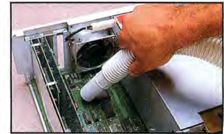
Photo 7. Vacuuming dust from inside surfaces.
