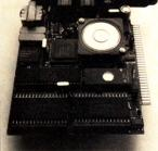
Novations' 2400 XE/HC half-card modem features automatic equalization.
