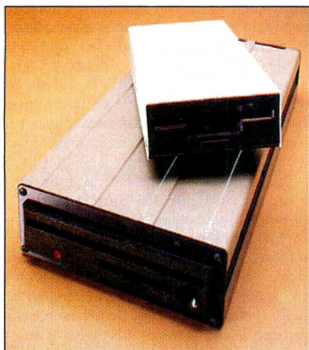
The Manzana MDP3T 3½-inch drive (top) and Pacific Micro Systems' Pelican 5¼-inch drive.
