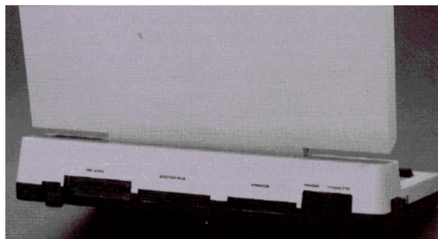
Photo 3. Relocation of the expansion bus to the rear of the computer makes connecting peripherals easier.
