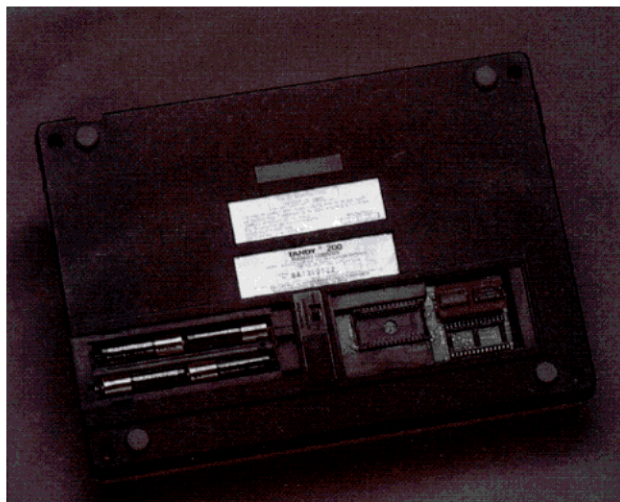
Photo 2. The Model 200's battery slot (left) takes two rows of batteries, and the 24K memory expansion modules are easy to put in place.
