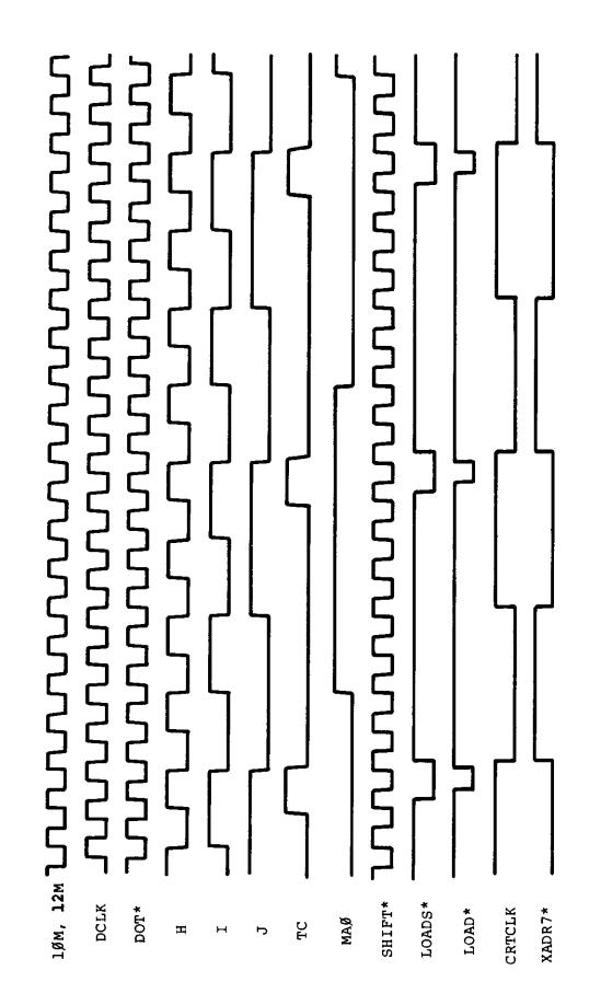
Figure 3-3. Video Timing 64 x 16 Mode 80 x 24 Mode
