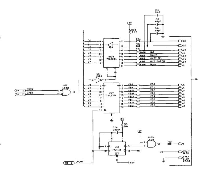
Figure 2-19. Printer Circuit
