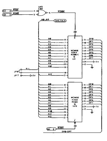
Figure 2-14. ROM Circuit (Page 1 of Schematic)
