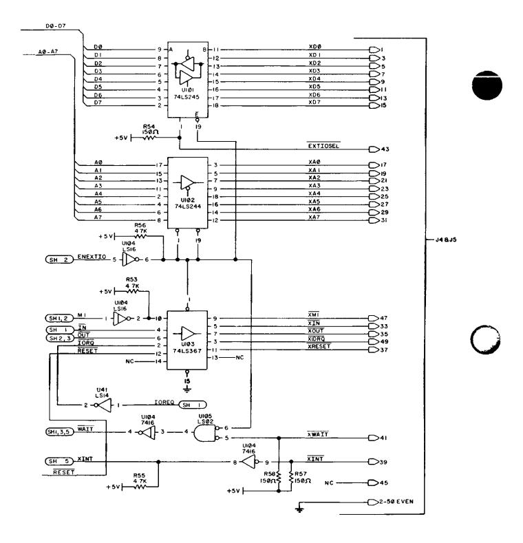
Figure 2-22. I/O Port (Page 4 of Schematic)
