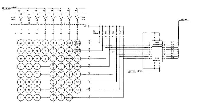
Figure 2-17. Keyboard (Page 4 of Schematic)
