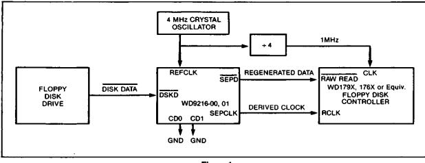
Figure 1. TYPICAL SYSTEM CONFIGURATION (51⁄4 " Drive, Double Density)
