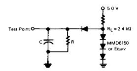
$\begin{array}{l} C = 130 \ \text{pF} \ \text{for} \ D0\text{-}D7 \\ = 30 \ \text{pF} \ \text{for} \ \text{MA0-MA13}, \ \text{RA0-RA4}, \\ DE, \ \text{HS}, \ \text{VS}, \ \text{and} \ \text{CURSOR} \\ \textbf{R} = 11 \ \text{k}\Omega \ \text{for} \ D0\text{-}D7 \\ = 24 \ \text{k}\Omega \ \text{for} \ \text{All} \ \text{Other} \ \text{Outputs} \end{array}$
