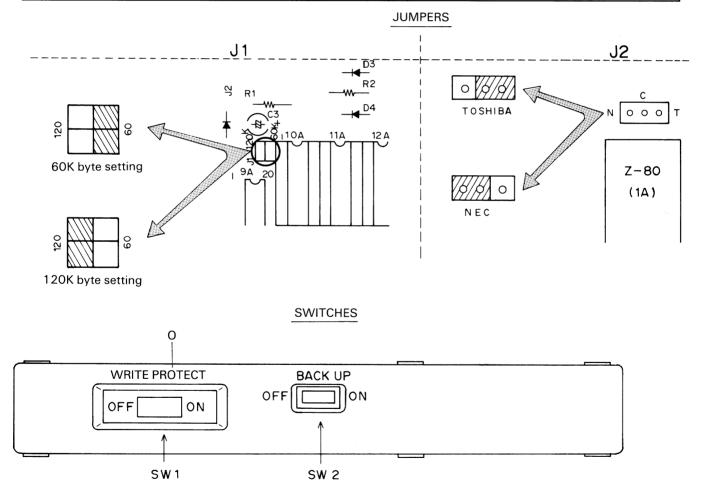
Fig. 3-31 Jumper and Switch Location
