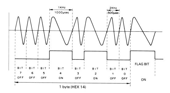
Fig. 3-18 Sample Write Signal Waveform
