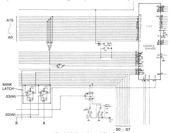
Fig. 3-38 Bank Control Circuit
