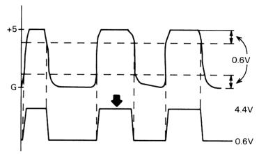
Fig. 3-19 Write Current Waveshaping
