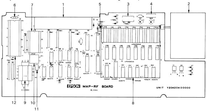
Fig. 3-29 RAM Disk Board Element Lay-Out
