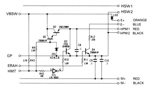
Fig. 3-12 Head Pinch Motor Control Circuit
