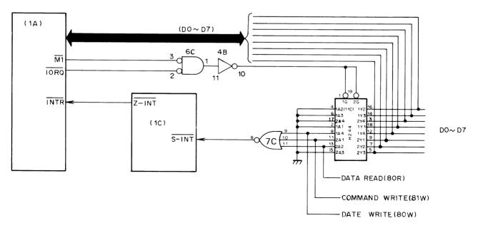
Fig. 3-39 RAM Disk Interrupt Circuit
