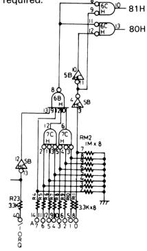
Fig. 3-34 RAM disk address decoder circuit
