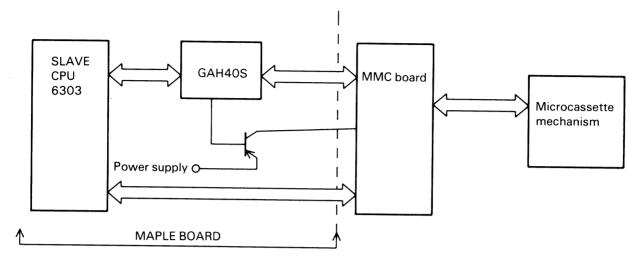
Fig. 3-1 Microcassette Tape Operation Control Block Diagram
