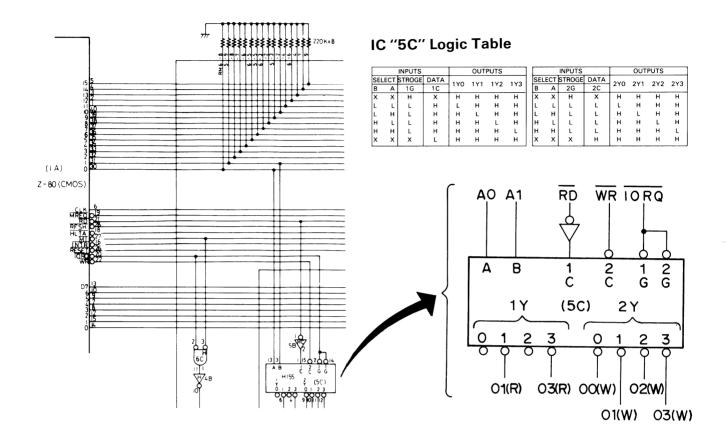
Fig. 3-37 I/O Selector Circuit
