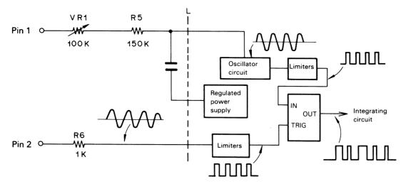
Fig. 3-8 Motor Speed Control Circuitry
