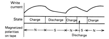
Fig. 3-14 Tape Write Current Waveform
