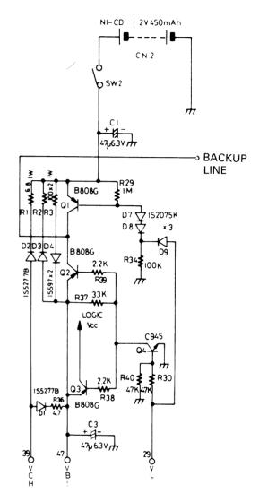
Fig. 3-32 Power Supply Circuit
