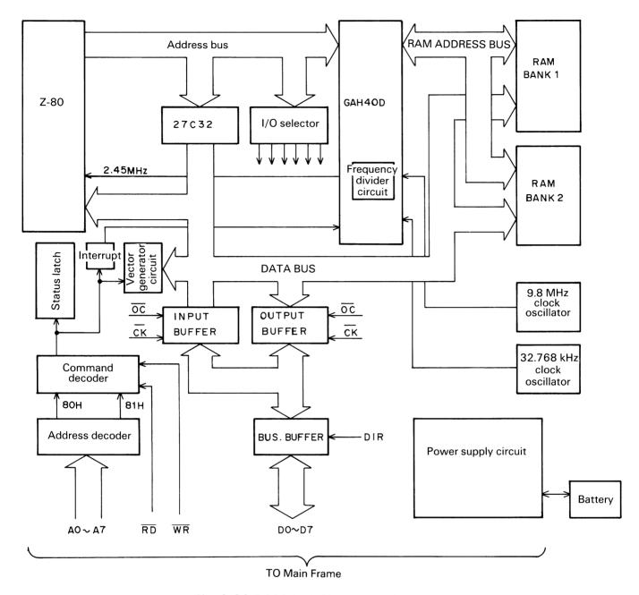
Fig. 3-30 RAM Disk Unit Block Diagram
