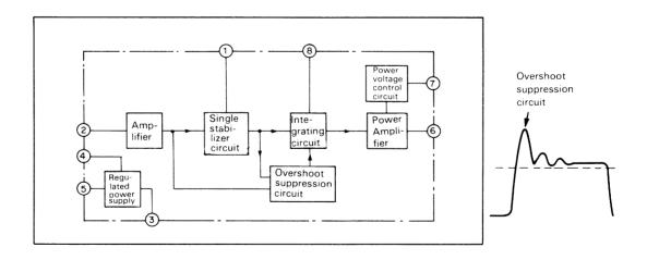
Fig. 3-7 IC2 Internal Circuit Block Diagram
