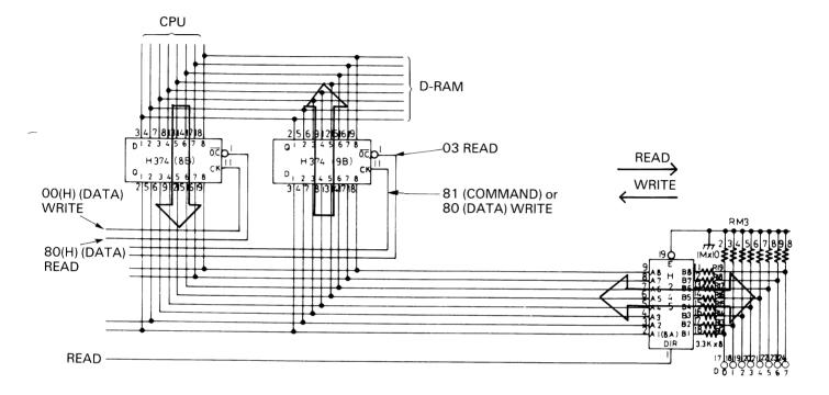
Fig. 3-36 Data Transfer Directions and Control
