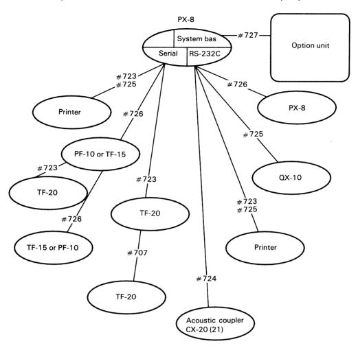
Fig. 1-8 Peripheral Device Information Cables
