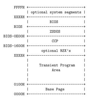
As depicted in the diagram, only addresses in the Base Page and the address of the start of TPA are fixed in a ZSDOS system. All other system address are calculated relative to BIOS. The sizes of ZSDOS, the Base Page, and the CCP are fixed. All other system segments may be sized as needed.
