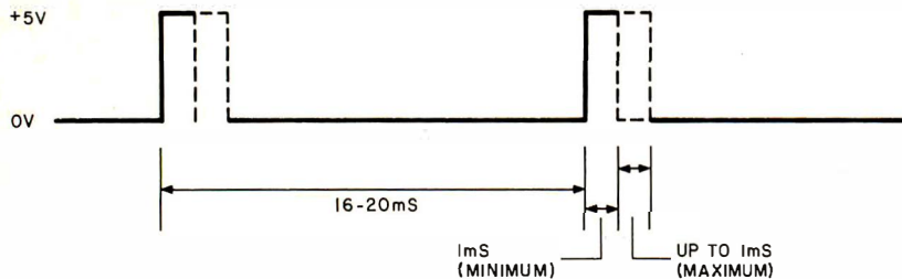
Figure 1: Timing diagram of the waveform that is needed to drive the servomechanism. The pulses are from 16 to 20 ms apart in time, and have a pulse width of 1 to 2 ms. This type of timing can be accomplished using your computer's internal clock as a reference in timing loops, or through a programmable real time clock.
